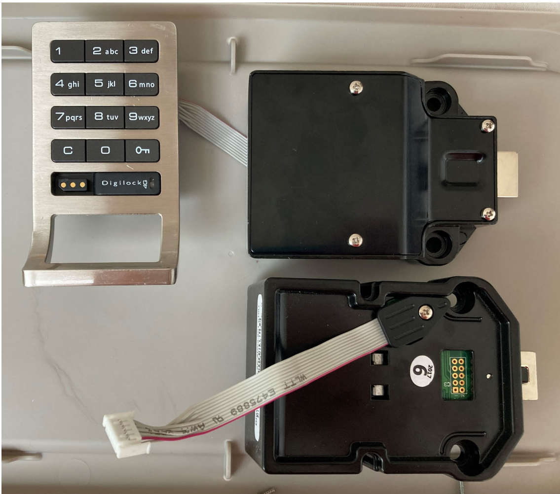
Digilock 4G (outside part) with latch unit (inside part)
