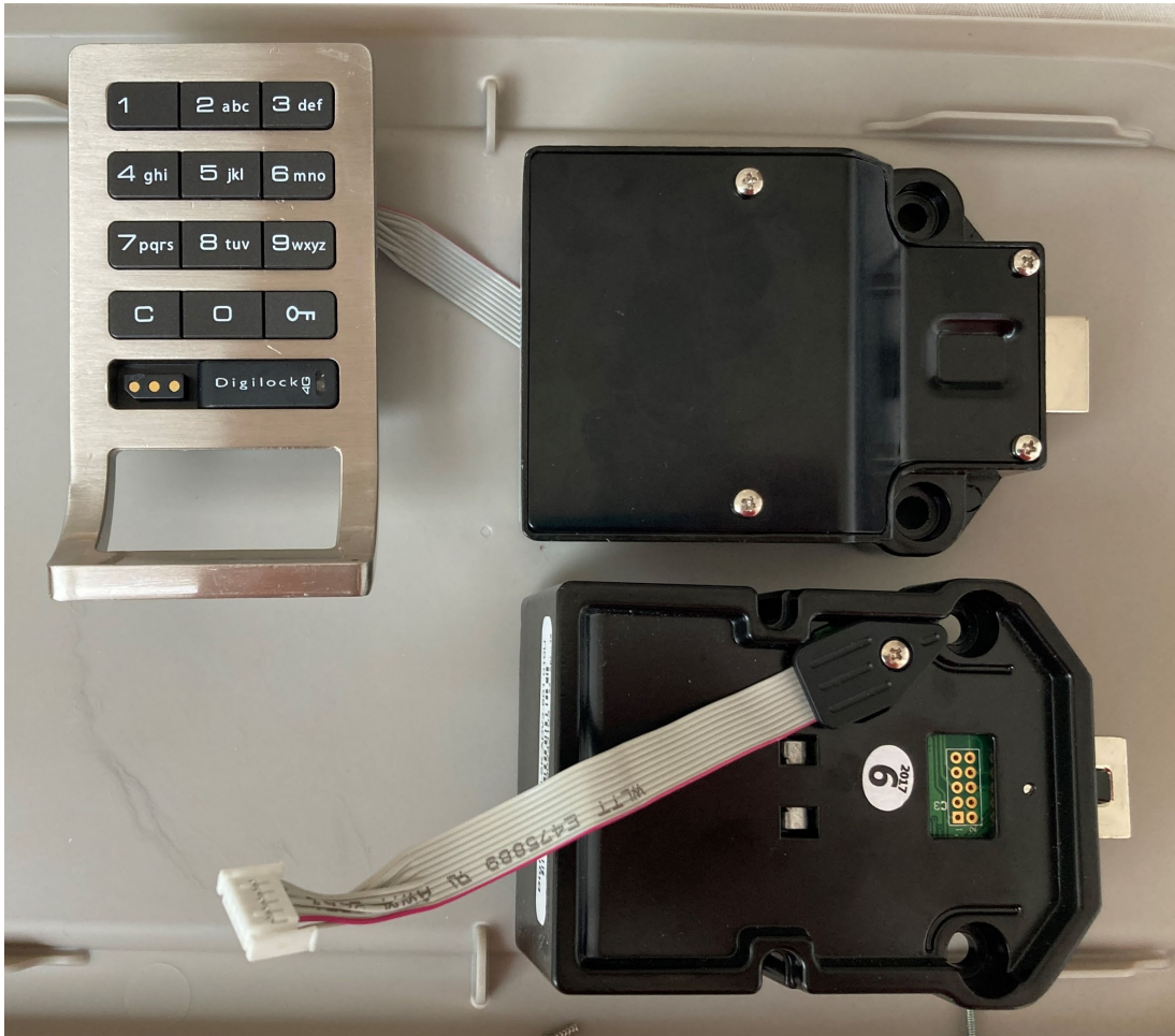
Digilock 4G (outside part) with latch unit (inside part)
